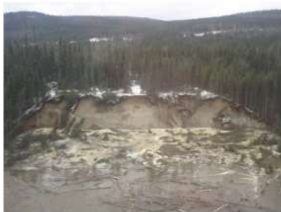
Figure 3-14: Landslides in a sandy bank with silt content at K.P 174,5 (Réf. H.-Q.-Polygéo-2007)
