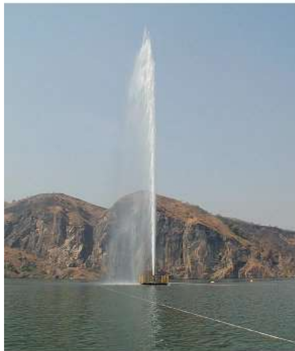
Figure 3-11: Degassing pipe in action
